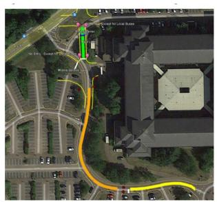
Figure 27: Indicative ketch of shuttle link showing bus link and signals locations
